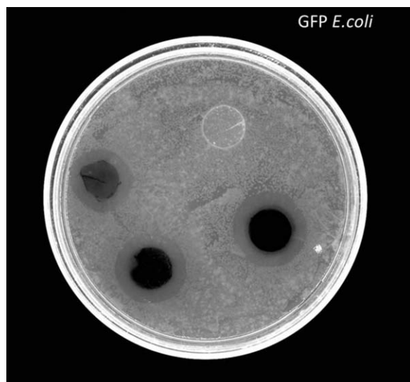
Figure 7. Antibacterial disc diffusion assay showing a zone of inhibition against Gram-negative recombinant GFP E. coli for 1, 2, and 3 wt % Ag composite nanofibers.
